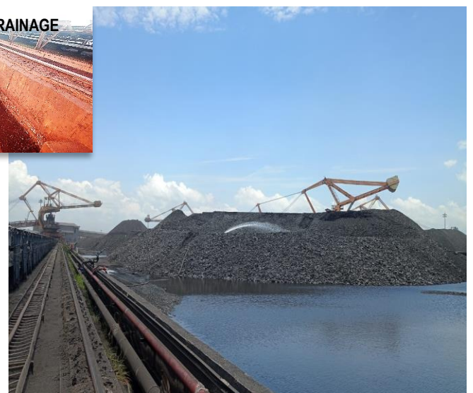
STACKER-RECLAIMER AND DUST SUPPRESSION SYSTEM IN OPERATION AT STORAGE YARD
